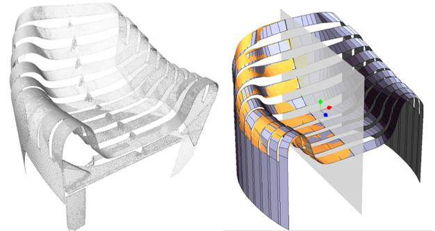
Fig. 16. 3D scanned data and extracted scanned data (orange) overlaid on the edited shape (blue).
