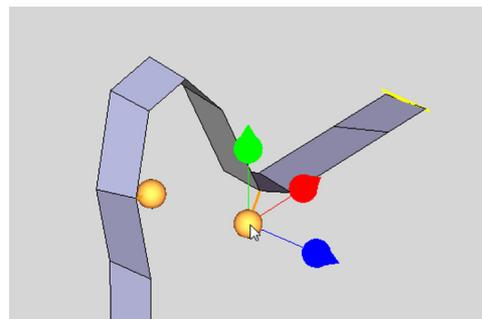
Fig. 12. Adding an anchor point (orange sphere) to a vertex.
