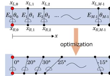
Fig. 3. Ridge lines before after optimization.
