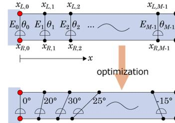
Fig. 3. Ridge lines before after optimization.
