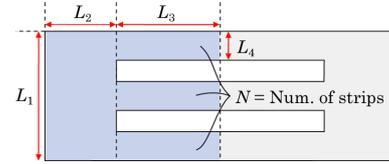
Fig. 2. Developed pattern defined by four numbers from  $L_1$  to  $L_4$  and number of strips  $N$ .
