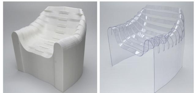
Fig. 17. 3D printed mold and the formed polyvinyl chloride board. Size(W/H/D): 247×233×179 mm.
